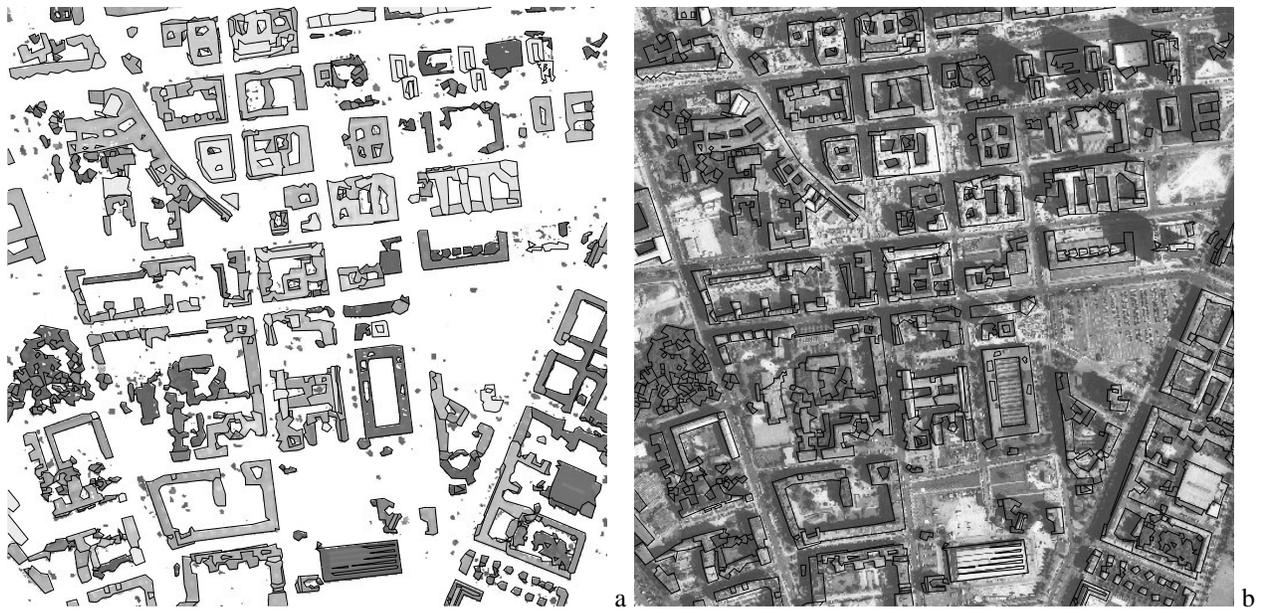
**Figure 5. Berlin results of automatic building extraction: (a) the polygonal approximation result superimposed on the DEM composed by all the extracted objects above the ground (small components are then discarded). (b) the final orthogonalized model superimposed on the ortho-image of the scene. Note that the model describes well the main structures of the buildings.**
