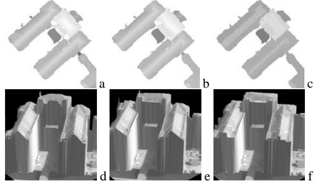
**Figure 2.** The pair of images (a and d) corresponds to the initial DEM and an arbitrary view of the building using this DEM and the ortho-photo, (b and e) corresponds to the synthetic DEM built using a segmentation in planar patches (22 patches selected) and (c and f) using the horizontal planar patches segmentation (11 patches selected).
