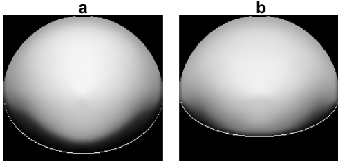
Figure 7. Spheres rendered using the BRDFs estimated from the bear model with (a) \theta_L = 45^\circ and (b) \theta_L = 60^\circ . The white lines indicate the calculated shadow boundary.
