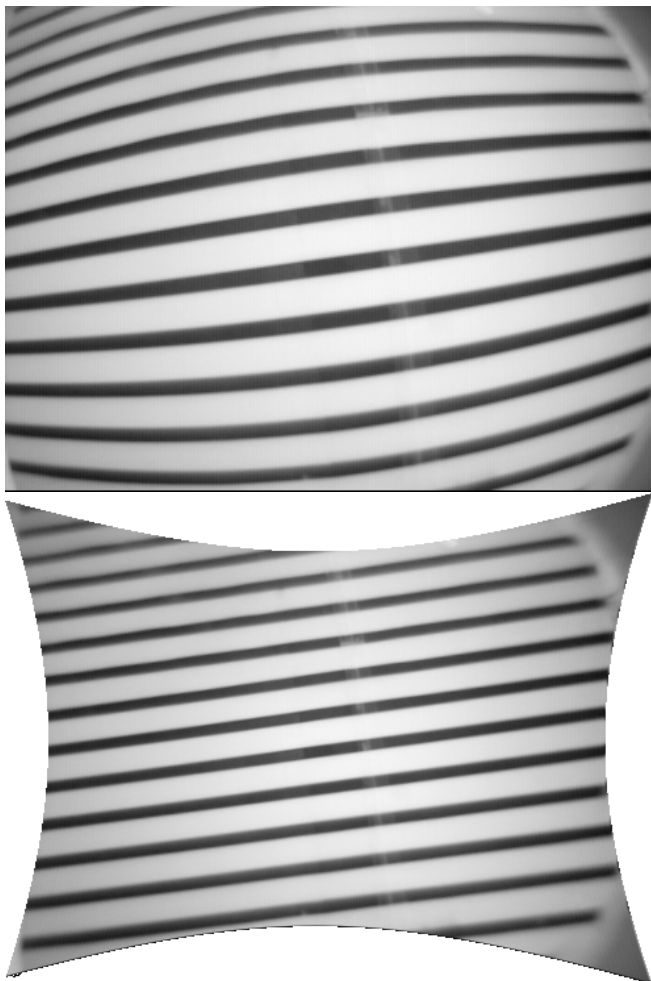
Fig. 6 An image taken with underwater fish-eye lens, and the same image undistorted using model 3^f . The parallel lines help checking the result of distortion calibration.
