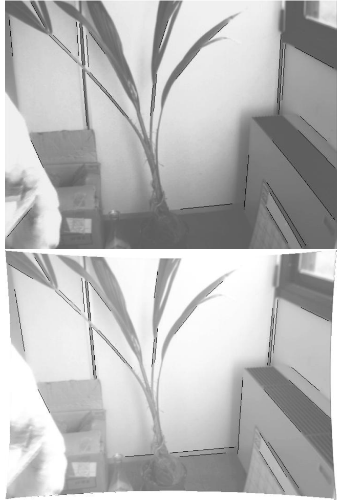
Fig. 5 A distorted image with the detected segments (left) and the same image at the end of the distortion calibration with segments extracted from undistorted edges (right): some outliers (wrong segments on the plant) were removed and longer segments are detected. This image represents the worst case, where some curves may be mistaken for lines.
