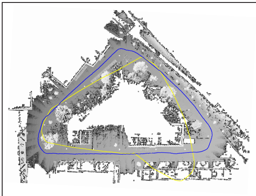
Fig. 7. MLS map used for the localization experiments. The area represented by this map spans approximately 195 by 146 meters. The blue / dark grey line shows the localized robot poses. The yellow / light grey line shows the pure odometry. The traversed trajectory has a length of 284 meters.
