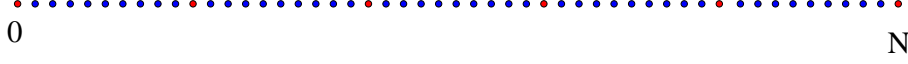
Figure 2: The repatoms (in red) are explicitly treated, all other atoms (in blue) being eliminated in the CG procedure.
