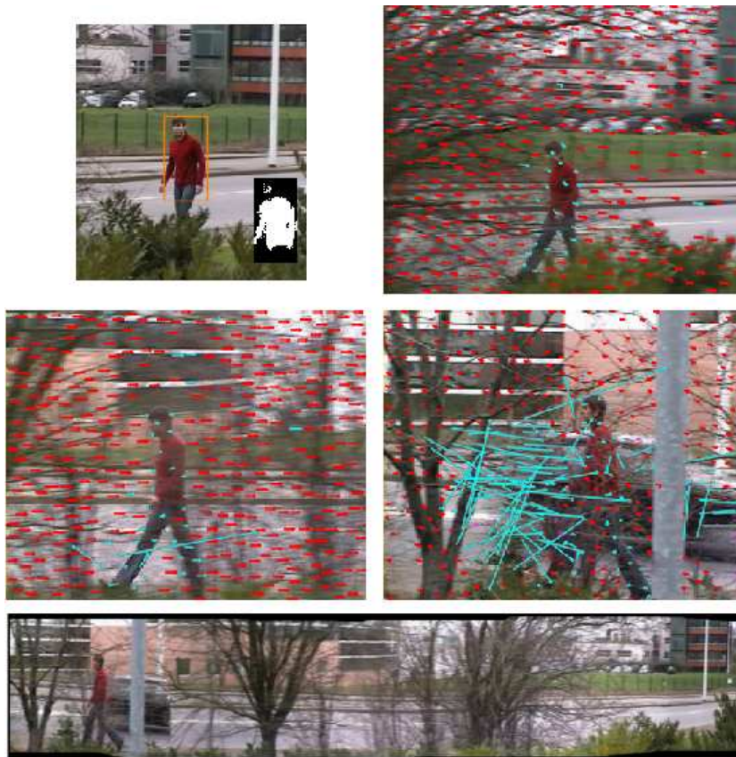
Figure 2: First image: background subtraction performed with the Bayes classification (the pixels selected are inside the orange rectangle). Images 2, 3 and 4: Background motion estimation. The red plots are inlier features and the blue ones are outliers, the lines are the corresponding flows. Bottom: Mosaic image reconstructed with the estimated camera motion.
