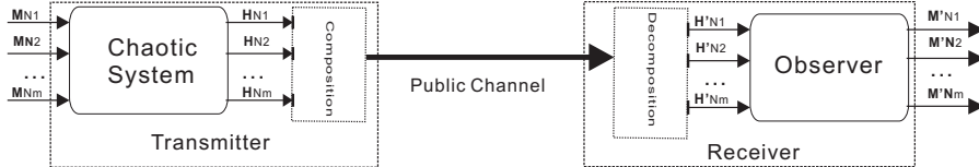
Fig. 1. Scheme for multiple secure communication system
