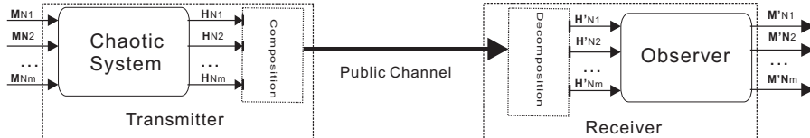
Fig. 1. Scheme for multiple secure communication system
