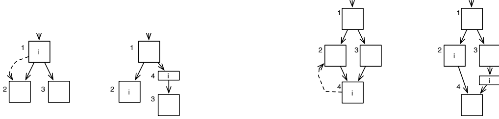
Figure 1. The two extra rules of trace scheduling. On the left, an example of move after a condition. On the right, an example of move before a join point. On each example the code is shown before and after hijacking.
