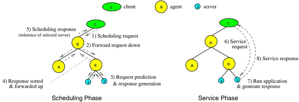
Figure 1: Platform deployment architecture and execution phases.
