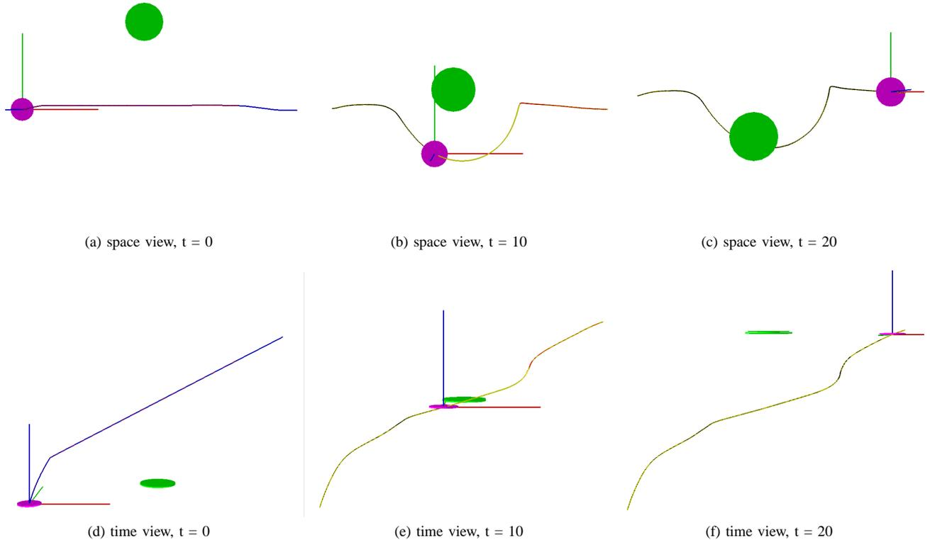
Fig. 4: Double integrator system, “cutting” scenario (spatial deformation):  $\mathcal{A}$  is moving from the left to the right, the obstacle is moving downwards. The top snapshots depict the path at different time instant ( $x \times y$  view). The bottom snapshots depict the velocity profile at the same instants ( $x \times t$  view).
