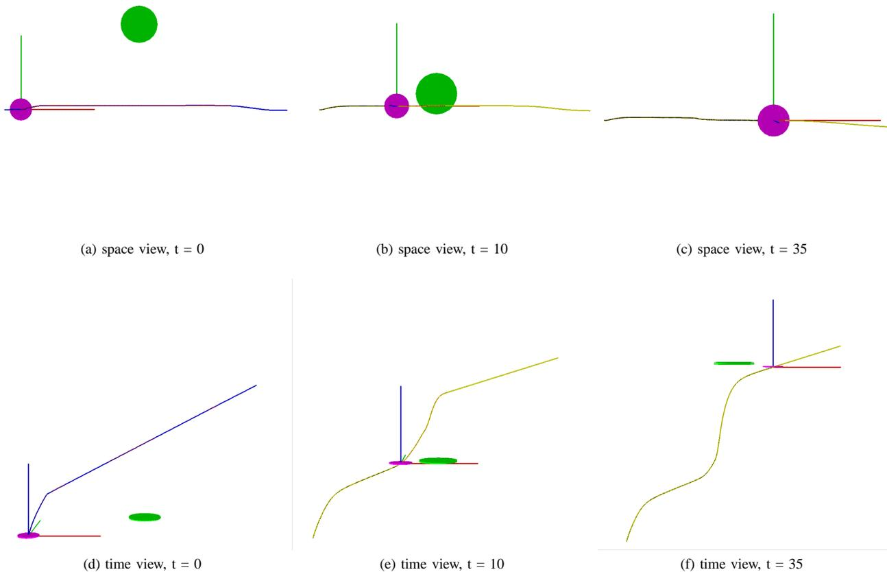
Fig. 5: Double integrator system, “cutting” scenario (temporal deformation):  $\mathcal{A}$  is moving from the left to the right, the obstacle is moving downwards. The top snapshots depict the path at different time instant ( $x \times y$  view). The bottom snapshots depict the velocity profile at the same instants ( $x \times t$  view).
