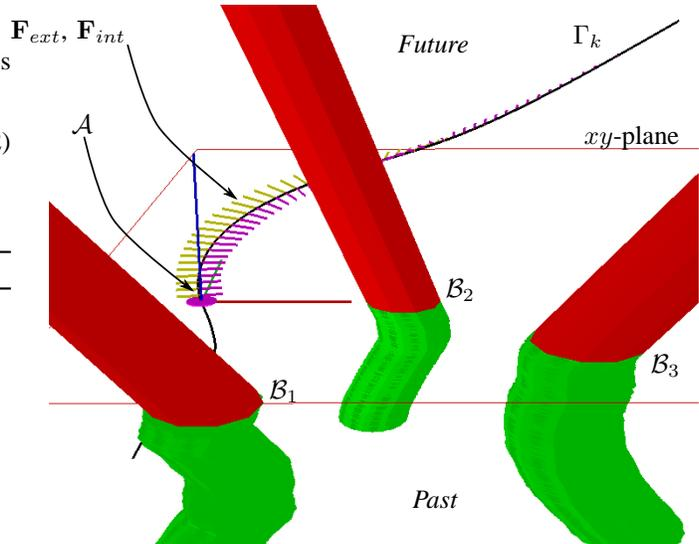
Fig. 3: Teddy's principle visualized in a scenario involving three moving disk obstacles  $\mathcal{B}_i$ ,  $i=1-3$ . The time dimension is pointing upward. The past lies below the  $xy$ -plane (the present) and the future lies above. The obstacles are moving randomly but the model of the future assumes that they maintain a constant linear velocity. The internal and external forces acting upon the nodes of the trajectory  $\Gamma_k$  are represented by vectors.
