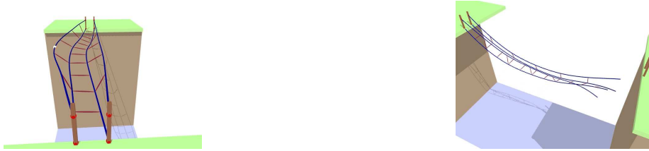
Figure 1: A bridge modeled with 4 deformable ropes, linked with distance constraints. Such constraints improve efficiency, maintaining realistic visual behavior.
