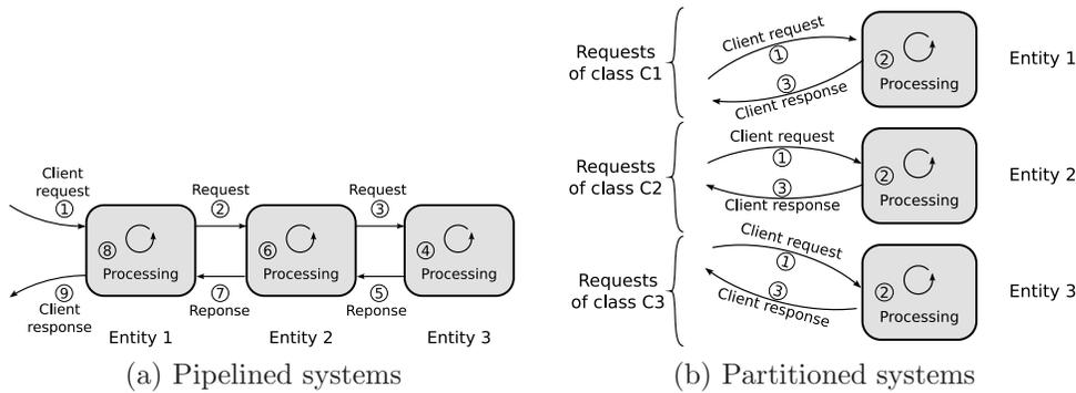
Figure 1: Application organization – pipelined versus partitioned systems
