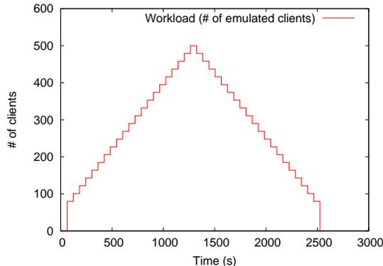
Figure 11: Generated workload to simulate gradual variations
