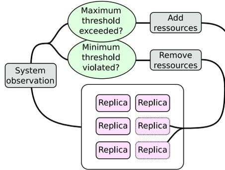
Figure 7: Dynamic provisioning control-loop and policy design
