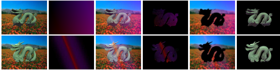
Figure 4: Synthesized dragon sequence. From left to right : 2 of 32 original images; components added for simulating the photometric camera effects; input images; estimated corrective component (scaled by 2 for visualization); estimated background images; estimated shape and radiance.
