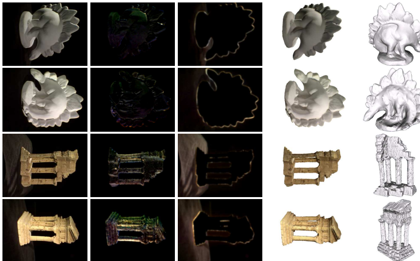
Figure 6: Dino and Temple sequence. From left to right: 1 of 16 input images; estimated non-Lambertian component (scaled by 8 for visualization); estimated background images (scaled by 2 for visualization); estimated radiance; estimated mesh seen from a different viewpoint.
