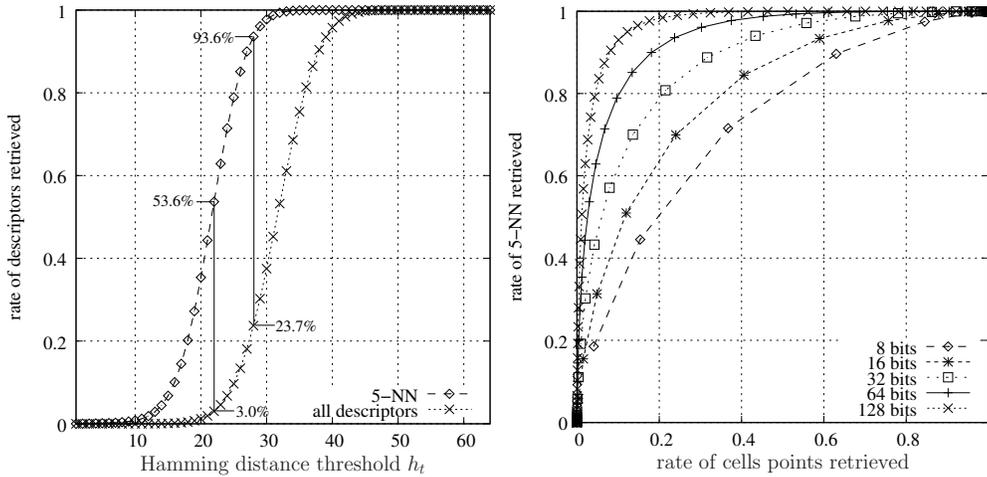
**Fig. 3.** Filtering effect of HE on the descriptors within a cell and on the 5 NNs. Left: trade-off between the rate of cell descriptors and the rate of NN that are retrieved for  $d_b = 64$ . Right: impact of the number of bits  $d_b$  of the binary signature length.
