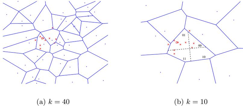
**Fig. 1.** Illustration of  $k$ -means clustering and our binary signature. (a) Fine clustering. (b) Low  $k$  and binary signature: the similarity search within a Voronoi cell is based on the Hamming distance. Legend:  $\cdot$ =centroids,  $\square$ =descriptor,  $\times$ =noisy versions of the descriptor.
