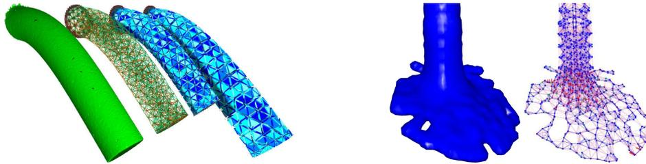
**Figure 4.** Left: surface of an actual soft cylindrical object compared to a mass-spring, co-rotational FEM, and linear FEM models, under the same constraints. Right: a fluid modeled in SOFA using a SPH method.
