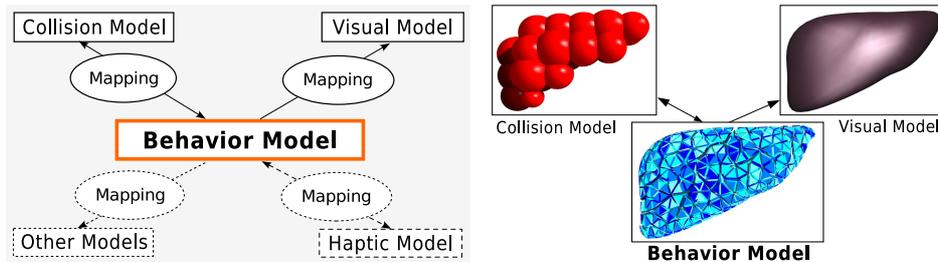
**Figure 1.** Illustration of the multi-model representation in SOFA. *Left:* possible representations for a simulated object, with the Behavior Model controlling the update of the other representations through a series of mappings. *Right:* examples of these representations for a liver model. Notice how the Visual Model is more detailed than the Behavior Model and how the Collision Model relies on a very different representation.
