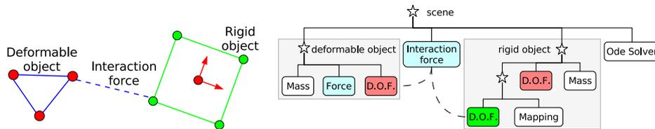
**Figure 2.** Left: two interacting bodies. The DoFs are shown as circles, and the forces as lines. A solid line describes an internal force, a dotted line an external force. Right: graph associated to the scene on the left. The nodes of the scene-graph, shown as stars, allow to model structured groups of components.
