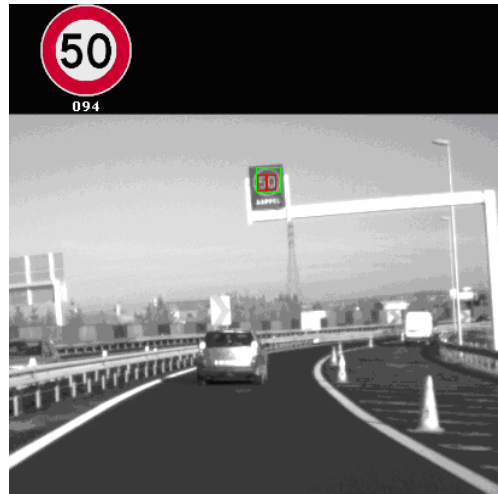
Fig. 10. Successful LED speed-limit sign recognition obtained with our system without specific re-training, by just inverting pixel scale inside region of detected circles.
