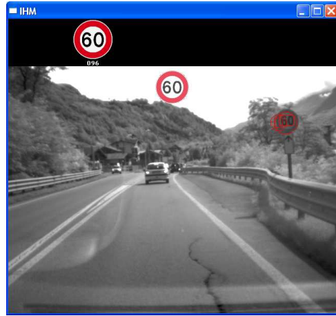
Fig. 9. Correct recognition of a Italian speed-limit sign illustrating promising results for pan-European speed-limit recognition.
