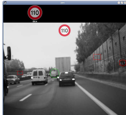
Fig. 8. Example of a tagged speed-limit sign correctly recognized thanks to our new global number segmentation
