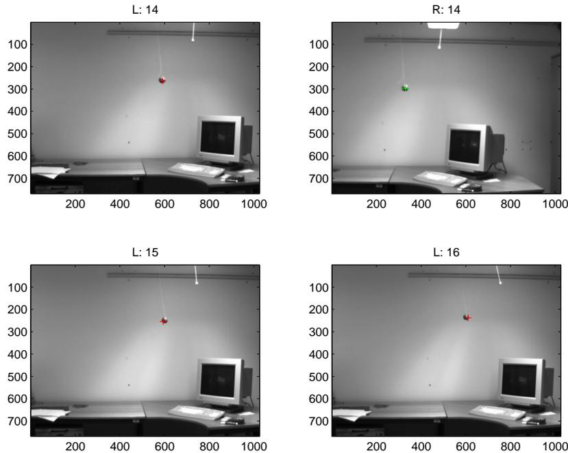
**Fig. 2.** The tracking result 14, 15 and 16 frames after the simulated sensor failure. The state (i.e. the position in the left image) is obtained by channel-based tracking given the measurements (i.e. the position in the right image). The cross in the upper left image is the estimated position at 14 frames after the simulated sensor failure given the measurement in the corresponding right image, upper right. The lower images show the estimated position after 15 and 16 frames.
