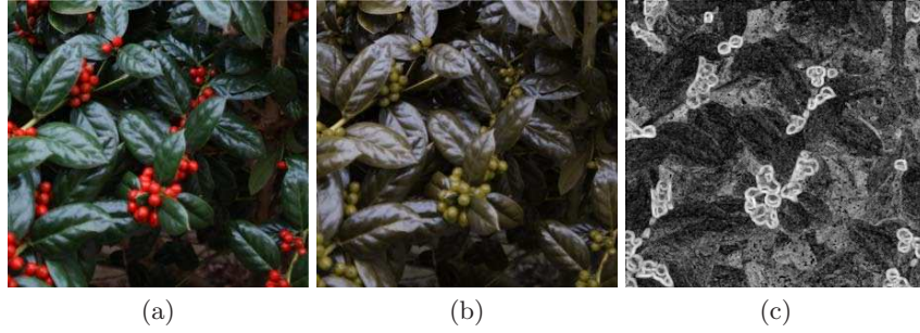
Fig. 2. The information loss map in image “berries”. (a) The original color image. (b) The simulation result for protanopia. (c) The local color contrast loss map in logarithmic scale.
