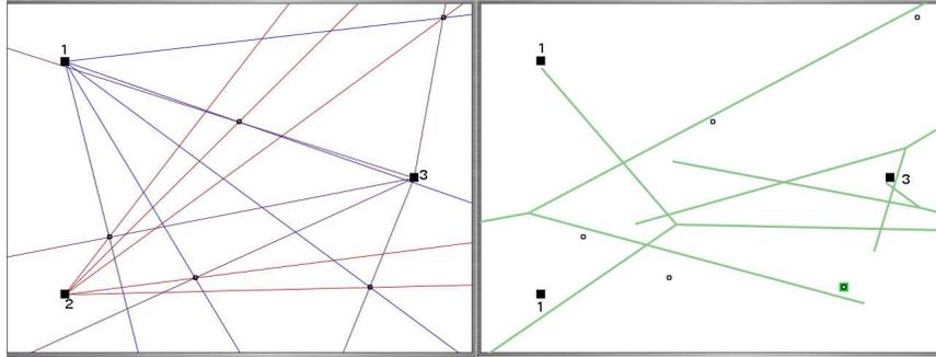
**Fig. 8.** Initial position with 3 cameras and 5 objects in simulation - *left*, LOS and objects - *right*, objects and Y shapes spanning the triangles of misclosure. The bottom right object is identified correctly at the start.
