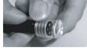
Fig. 4. Omnidirectional vision attachment positioned at the tip of an endoscope.
