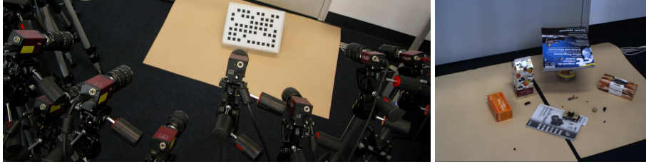
Fig. 5. Setup of the real experiment. Left: the multi camera system observing the pattern for the Zhang calibration, right: the scene (image from the sixth camera).
