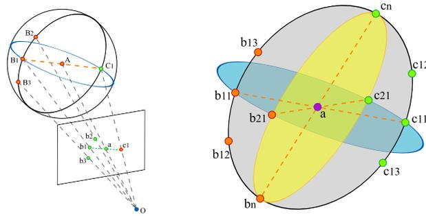
Fig. 1. (Left): The spherical calibration object; (right): image of a globe.
