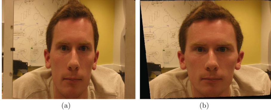
**Fig. 6.** a) Face image from flexible mirror imager after  $12\text{mm}$  deflection; b) Near-perspective face image with non-linear distortion removed using calibration data. Note the large distortion at top right of the image that was not captured by the calibration
