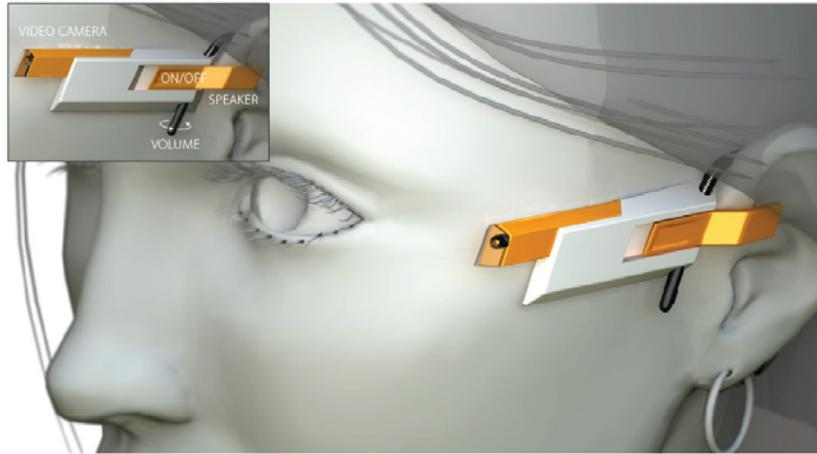
**Fig. 3:** An ear-mounted video camera and sound emitter
