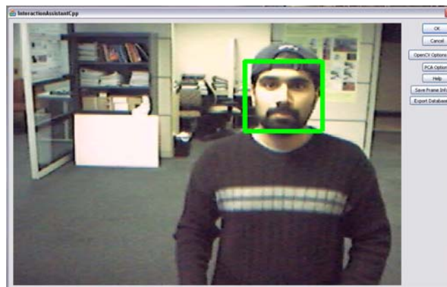
Fig. 7: Screen shot of the demonstration software performing face detection; image captured from the camera on the prototype hardware.
