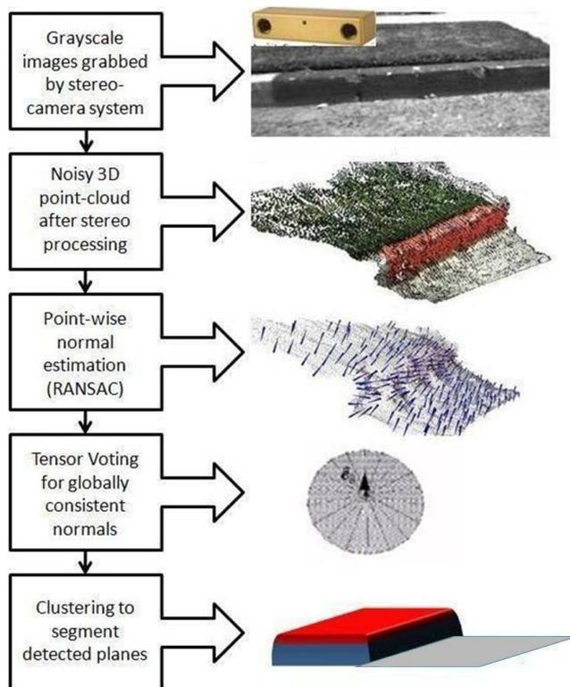
**Fig. 1.** Block diagram of our piecewise planar modeling algorithm. The stereo camera generates a dense 3D point-cloud, to which we fit normals by RANSAC. These normals are globally inconsistent because they are the result of local processing in each voxel of data. Tensor voting is employed to refine these normals and clustering is finally performed to segment out the fit planes
