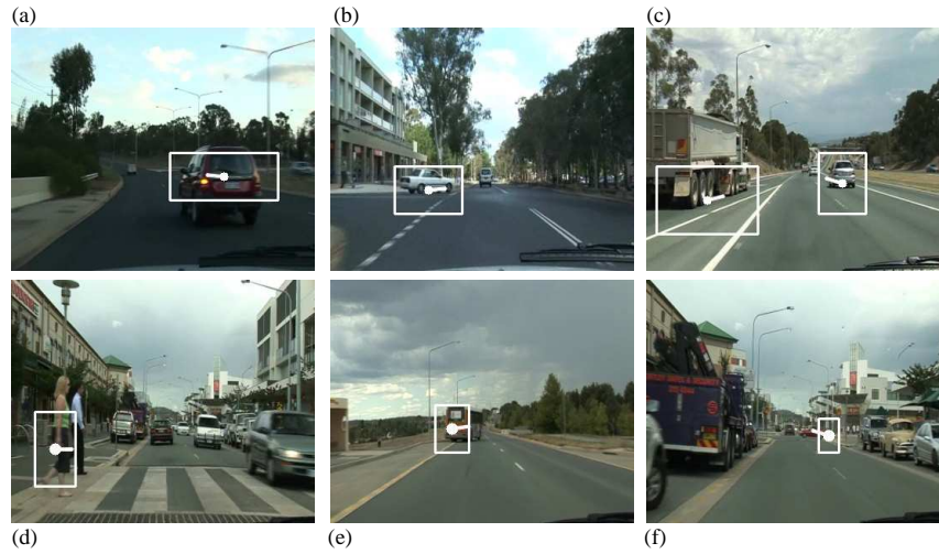
Fig. 3. Sample hazard detections from video segment (vs) testing: (a) merge from right (vs 1, 29.36 sec), (b) car turns out from left (vs 1, 52.79 sec), (c) truck merges from left (vs 1, 271.45 sec), (d) pedestrians crossing (vs 5 101.78 sec), (e) bus pulls out from left (vs 6 166.93 sec), (f) car crosses road from right (vs 5, 109.84 sec)
