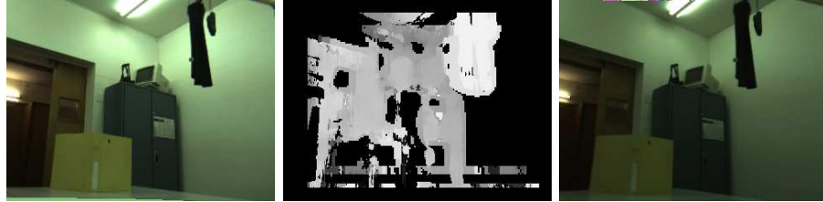
Fig. 5. Images of the left (left) and right (right) views of the stereocamera, and the resulting disparity map (centre). On the disparity map, the lighter the closer. A zero value (black) means that the distance is undetermined for that pixel.
