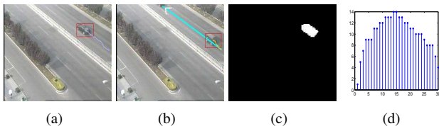
Figure 4. Motion features of a vehicle. (a) A vehicle is detected. (b) The direction of motion of the vehicle. (c) The binary mask of the vehicle. (d) Vertical projection histogram of the vehicle, the number of bins is the width of the vehicle.
