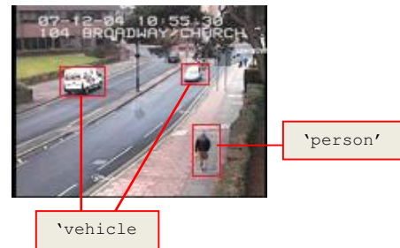
Figure 8. Initial tags/labels from Low Level Object Detector.
