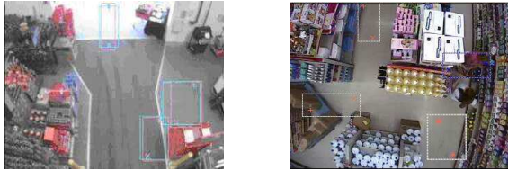
Figure 6: Visual verification of calibration accuracy: (a) user specified (blue) and corresponding computed (pink) features; (b) user specified calibration features (white) and computed features (dark blue) superimposed on a human target not used during calibration
