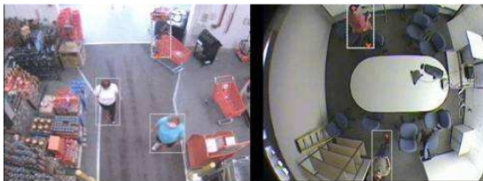
Figure 5: Calibration images: 3 features (bounding box, head, foot) marked on each target used for calibration
