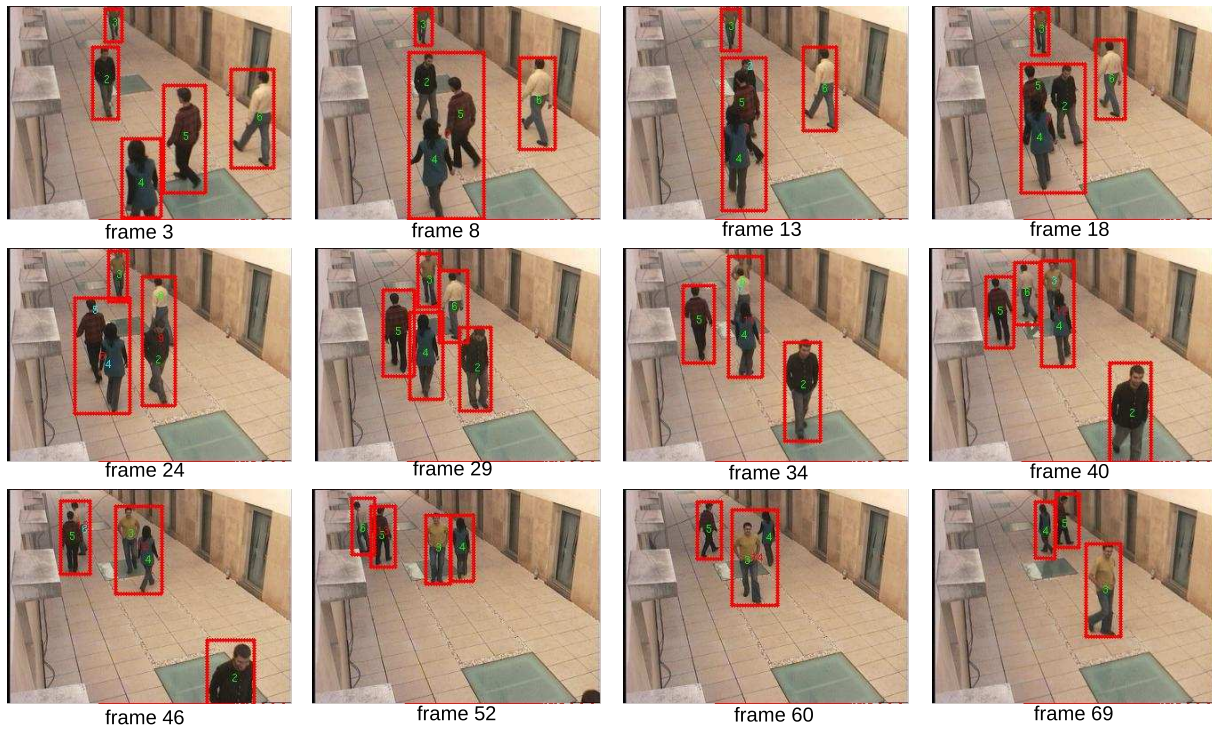
Figure 6. Results of a scene with five people that occludes each others; the red numbers means a group object; the single objects are represented with the green numbers; the cyan numbers means a estimate based only on the model dynamics, the red rectangles shows the blob region.
