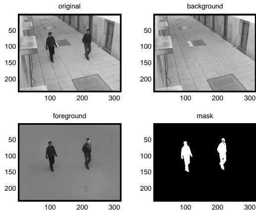
Figure 2. Segmentation process results - upper left is the original image, upper right is the background image, lower left is the foreground image and the lower right is the mask image.
