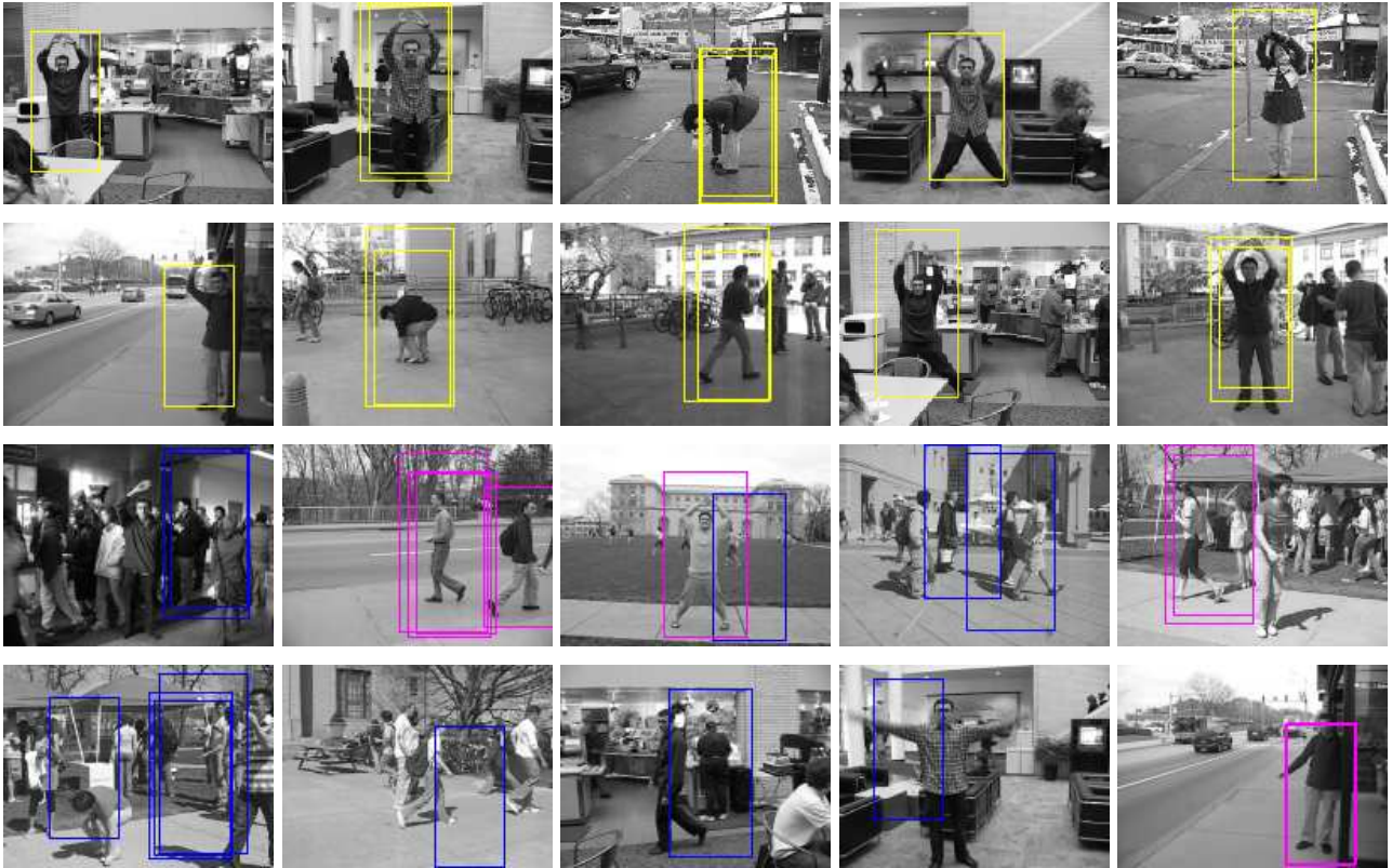
Figure 8. Tests with a 200 stump classifier in scenes with complex background. First two rows, examples of correct detection and classification (yellow). Last two rows, examples of misclassification (magenta) and false positives (blue).
