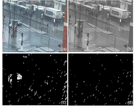
Figure 11. (a) Original rainy image; (b) BG model; (c) FG model; (d) resulted rain streaks.
