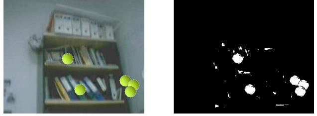
Figure 2. Synthetic sequence. Left: input image; Right: segmented image.
