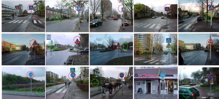
**Fig. 5.** Sign detection over 5 sample test images. Top row: pedestrian, middle: crossing, bottom: bike. Red circle is the first attended location and yellow one is the second.
