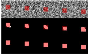
**Fig. 2.** Segmentation with temporal constraints. From top to bottom: (1) Input sequence (with groundtruth overlaid); (2) Segmentation results from regular 3D MRFs with appearance-based observation model (544 pixels misclassified); (3) Results from spatio-temporal MRFs with reliable temporal constraints induced by optical flow (32 pixels misclassified). From left to right: #1, #3, #5, #7, #9 out of the total 9 frames.
