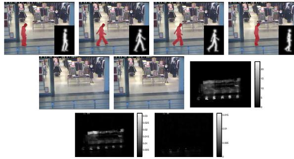
**Fig. 4.** From top to bottom: (1) Input sequence with output overlaid and the estimated shape prior shown in the bottom right; (2) Initial and re-estimated background models and their difference; (3) Variances of the initial and re-estimated background models.
