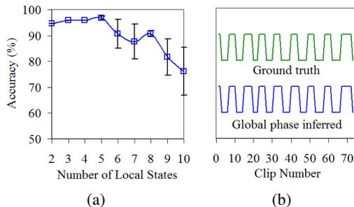
**Fig. 5.** (a) The matching accuracies of global traffic phases inferred from training data with the ground truth global phases averaged over ten runs, along with the standard deviations being shown as error bars. (b) Global phases inferred from training data and the ground truth global phases.
