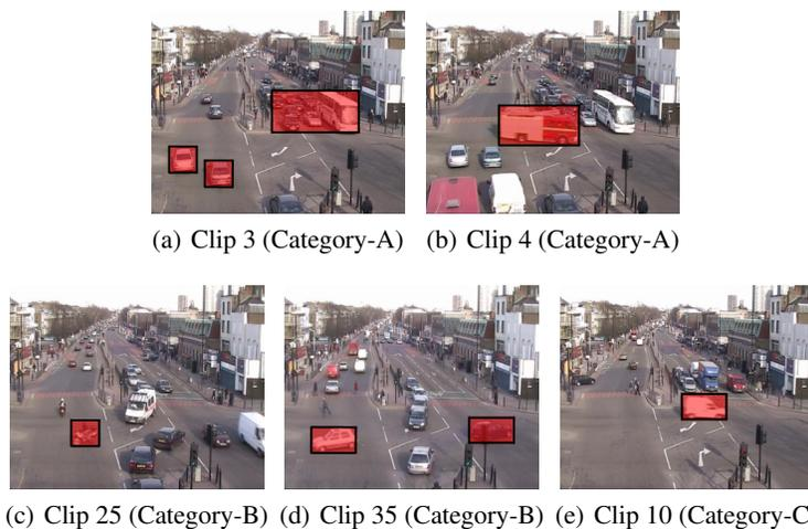
**Fig. 4.** Clips 3 and 4 are abnormal behaviours that are visually detectable (Category-A), whilst clips 25 and 35 are abnormal behaviours that are ambiguous (Category-B). Clip 10 contains subtle anomaly that is almost undetectable by human (Category-C). The corresponding objects that caused the anomalies are manually highlighted.
