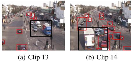
**Fig. 7.** Imperfect blob detections result in local atomic events being grouped into wrong clusters. The corresponding bounding box is marked in black colour.
