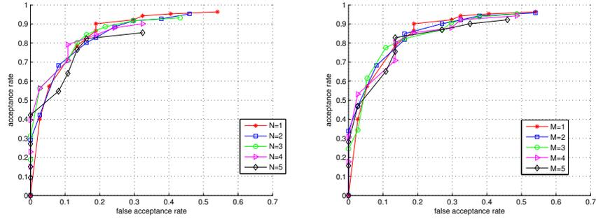
**Fig. 8.** Strategies to associate a single feedback to a video. Left: multiple peak (acceptance if  $N$  confidence values are above  $T_1$  — see text). Right: running average (acceptance if the average of  $M$  consecutive values is above  $T_2$  — see text). ROC curves are build varying  $T_1, T_2$  between 0.1 and 1.
