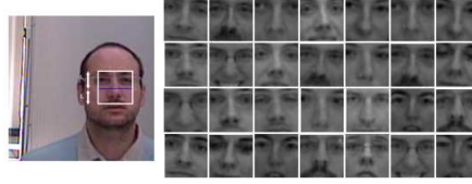
Fig. 4. Face registration: on the left, the areas considered to form the new registered face. On the right, examples of automatically registered faces.
