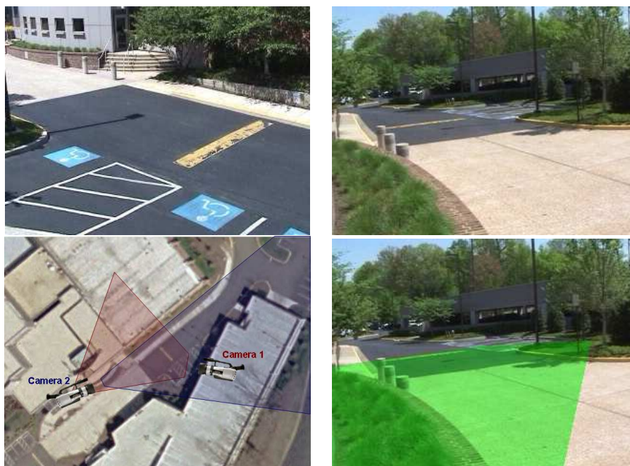
Fig. 6. Unsupervised alignment of visual sensors with overlapping fields of view: (Top Row) Camera views, (Bottom Left) Camera Setup (Bottom Right) Warped Image using the homography estimated from only 5 minutes of target observations.
