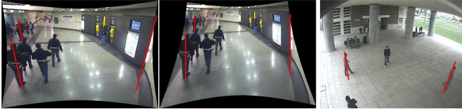
**Figure 1:** Vertical vanishing point mapping. *Left:* after distortion removal and before the mapping. We can observe people slant according to their position. *Central:* after the mapping to the infinity. Bounding-boxes will fit more closely the silhouette of people. *Right:* another example.
