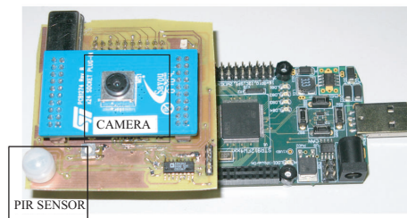
Fig. 2. Developed prototype of the video sensor node.
