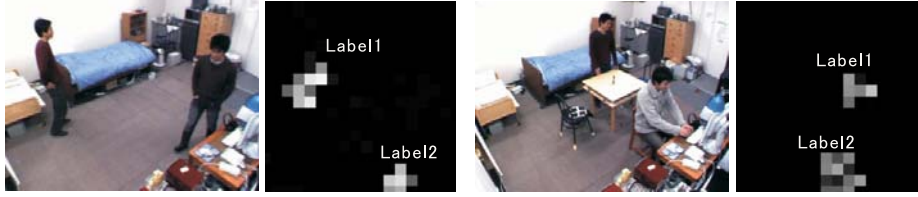
Fig. 2. Weight on floor sensors
