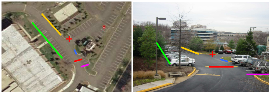
Figure 3: Selecting matching features. In this corresponding pair of map (left) and view (right), it is much easier to find matching lines than points. Matching features are represented by the same color.
