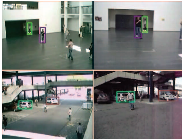
Fig. 1. Left column: objects of interest highlighted in a fixed camera. Right column: objects detected and matched by the proposed approach in a mobile
