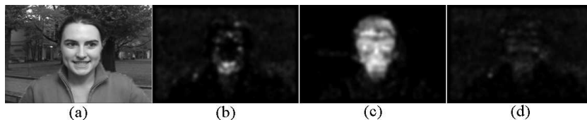
Fig. 2. Audiovisual correlation using different optical flow elements. The whiter a pixel, the higher its correlation. (a-d) show the original image, correlation by horizontal element, vertical element and mode, respectively.
