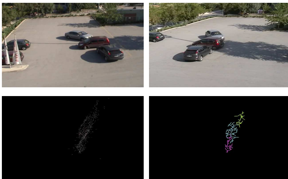
Fig. 3: Simulation results of occlusion handling from left to right and top to bottom, first input image, second input image, from the top-view transferred segment centers, clustered minimal spanning forest
