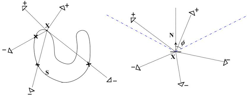
**Fig. 1.** Two approaches to visibility approximation (Lempitsky et al. [6]). On the left is a *state-based visibility*, the visibility information of a point  $\mathbf{X}$  with respect to all the views is determined by the current global scene geometry  $\mathbf{S}$ . On the right is an *oriented visibility*, a local patch  $(\mathbf{X}, \mathbf{N})$  is considered visible from the viewpoints within a predefined angle  $\phi$  from the normal direction  $\mathbf{N}$ .
