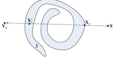
**Fig. 3.** Ray Tracing. A point is considered invisible to the viewpoint only in two cases. The first case is that it lies inside the scene surface and therefore it is occluded by the scene surface. The second case is that although it lies outside the scene surface, it is still occluded by another point before it in the same radial direction.  $\mathbf{X}'_1$  is invisible to  $\mathbf{V}_0$  in the first case and  $\mathbf{X}_1$  is invisible to  $\mathbf{V}_0$  in the second case.
