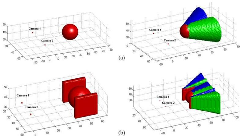
**Fig. 6.** Visibility results of two cameras applied to the synthetic scene with known geometry. The red surface represents the scene (occluders). The green and blue surface represent the boundary between visible and invisible regions to camera one and camera two respectively. (a) The visibility results of two cameras in a simple sphere scene. (b) The visibility results of two cameras in a scene with more complex geometry.
