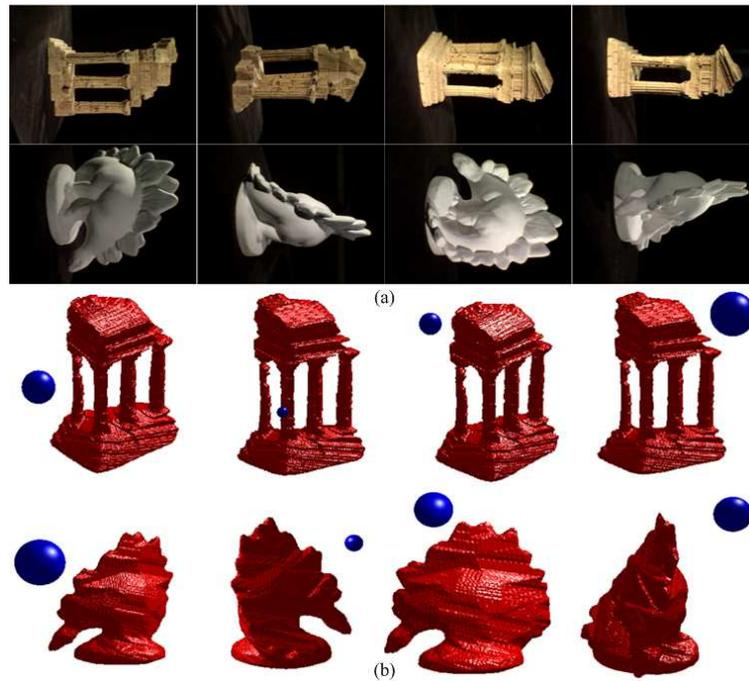
**Fig. 7.** The reconstruction results. (a) Some views of the *dinoSparseRing* and *templeSparseRing* datasets. (b) The reconstruction results of *dino* and *temple* (shown in red) with several different initializations (shown in blue).
